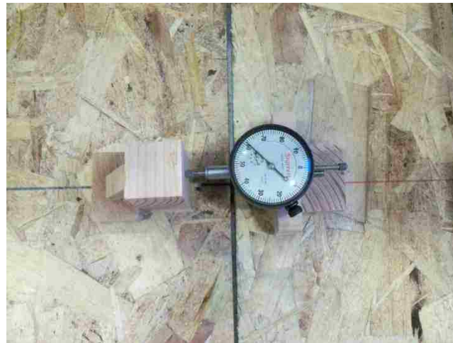
Figure 3.26 Dial gage installed at the gap discontinuity.
