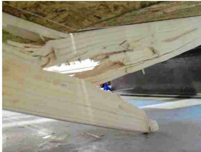
Figure 3.11 Failure of T-beam at a knot close to the gap in the OSB.
