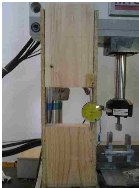
Figure 3.16 Specimen for testing connection behavior.
