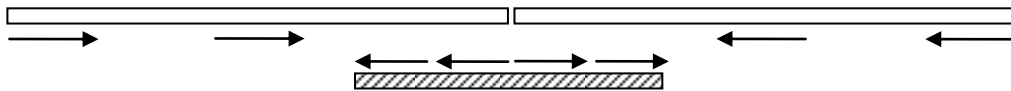
Figure 6.6 Free-body diagram of forces acting at the flange and at the added panel to provide continuity.
